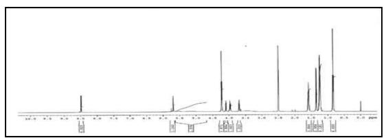
HPLC Purity ~98%; Mass: ES<sup>+</sup> 474.21 Figure No.6: <sup>1</sup>H NMR of the Di-Pentyloxycarbonyl Capecitabine
